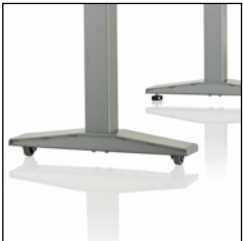
The rolling base option uses inline casters beneath one end of the table to allow a user to lift the opposite end and steer the base out of the way.
