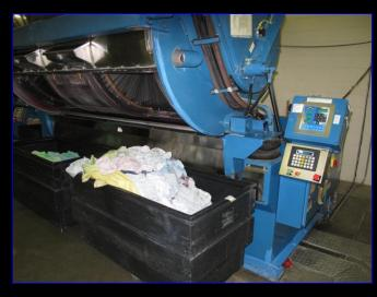
Large capacity washer extractors that are microprocessor equipped allow for precise control of all wash processes to insure consistent high quality results.
