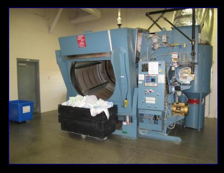
Patented axial flow dryers utilizing moisture sensors that are microprocessor controlled provides a safe drying environment for all fabrics.
