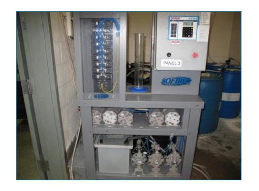
Proof of delivery confirmation on our networked, flow meter equipped chemical delivery system ensures that all loads receive the designed amounts of chemistry.
