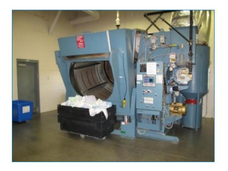
Patented axial flow dryers utilizing moisture sensors that are microprocessor controlled provides a safe drying environment for all fabrics.
