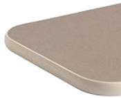
B. Perfect Edge: Made of 1/4" thick by 3/4" high cast black polyurethane. The Perfect Edge is mechanically and chemically bonded to the table core and chemically bonded to the laminate surface edge, providing a superior, permanently sealed barrier to moisture, dirt and bacteria penetration.
